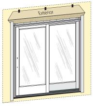
NOTE: Press all flashing tape down firmly.
