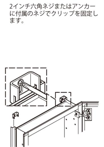
**11** Install the side brackets. Remove the backing.
