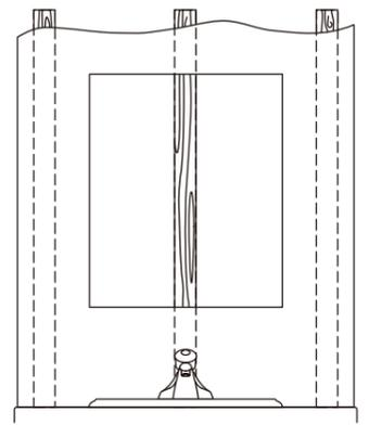
**4** Frame out the wall cavity.
