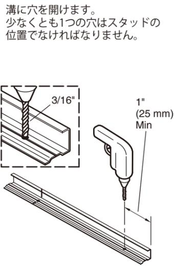
**4** Mark hole locations on the wall. Drill holes. Insert anchors (not provided) where needed.
