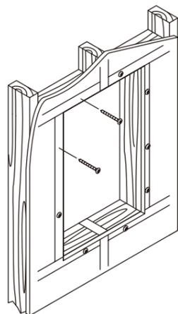
**6** If applicable, rotate the cabinet for a right or left door swing.
